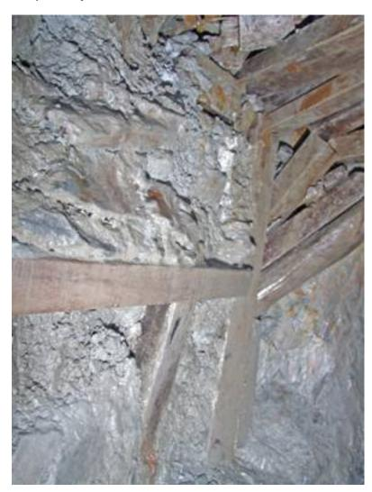
Turning right and following the fault I had to put a lot of timber in. Just in front the roadway inclines down. As we drove our roadway, we had been gradually climbing.
