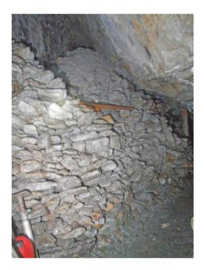
All of the packwork shown on the left is material extracted from our digging operations. Eventually, we ran out of room to tip, and had to start dumping in the engine winze. The way on is seen middle right past the timber prop.
